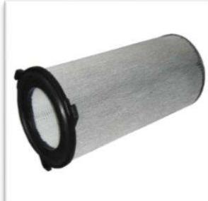
The filter cartridges are made of pleated polyester fabric, with the application of powdered aluminum that ensures the removal of electric charges, created by the dust filter. The issue of dust is less than 0.1%, grain size between 0.2 and 2 microns. The filter cartridge has an excellent resistance to organic solvents, and has a maximal temperature of use in continuous operation of 150 ° C. Its particularly smooth surface allows an optimal detachment of the powder.
